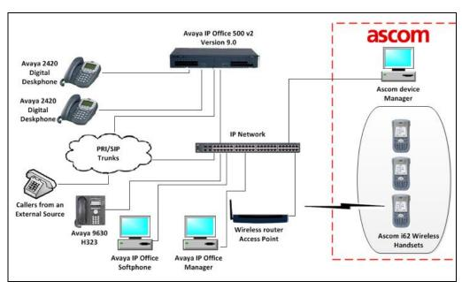
Figure 1: Avaya IP Office and Ascom Reference Configuration
