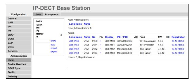
The Ascom DECT handset connection to Session Manager can also be verified by an absence of an error message on the handset display as shown in the following illustration, (note this is an example from compliance testing).
