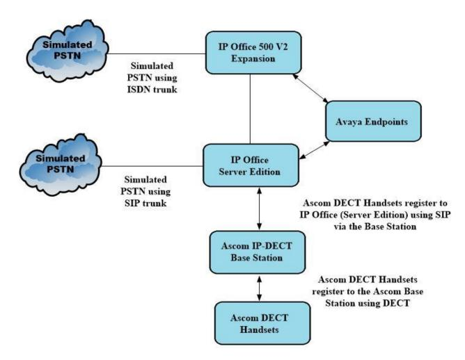
Figure 1: Avaya IP Office and Ascom Reference Configuration
